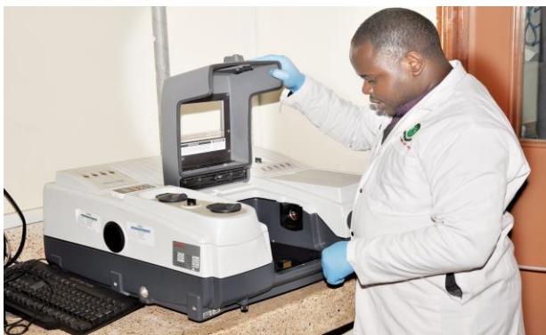
Fourier transform infrared spectrometer: Used for identification of medicines.
