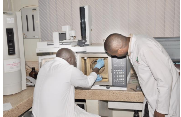
Gas chromatography equipment, used for testing insecticides in the LLINs and acaricides.
