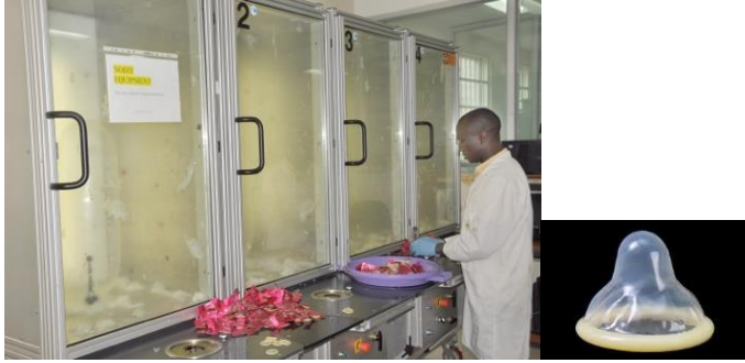
Condom Air Burst equipment: Tests for air pressure and volume of the latex condoms.
