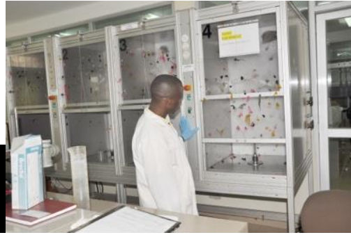
Condom Air Burst equipment: Tests for air pressure and volume of the latex condoms.
