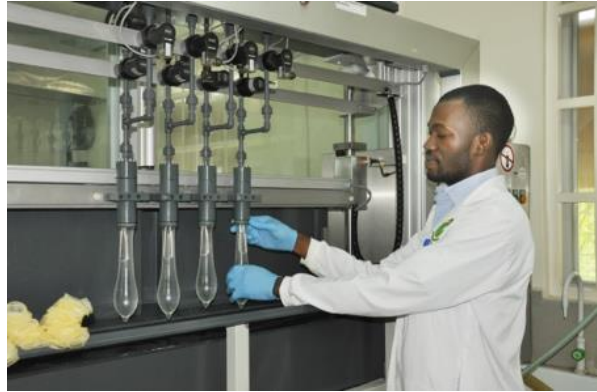
Condom Air Burst equipment: Tests for air pressure and volume of the latex condoms.
