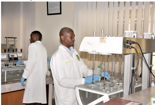
Dissolution testers used for testing the amount of medicine that dissolves in the body.
