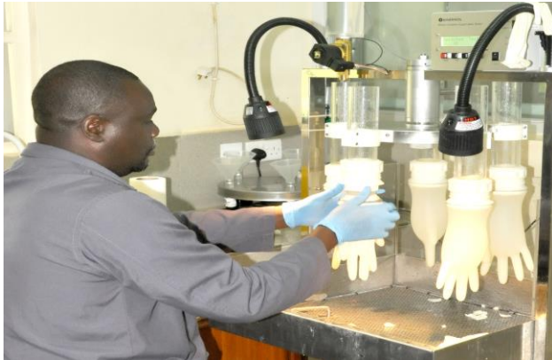
Gloves/ Condom visual leak tester: used to ensure that medical gloves are free from holes.
