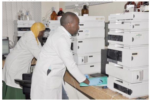
High performance liquid chromatographic systems (HPLCs). NDA has state of the art fully automated equipment and technical expertise with vast years of experience in the analytical area, dedicated to doing routine testing of all medicines in Uganda.
